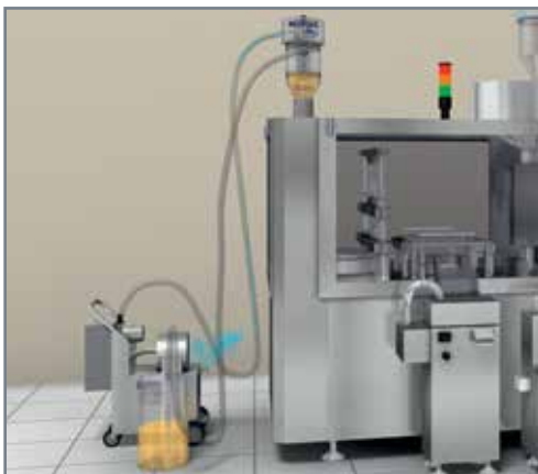
Powders are conveyed in selected quantities and within desired time.
